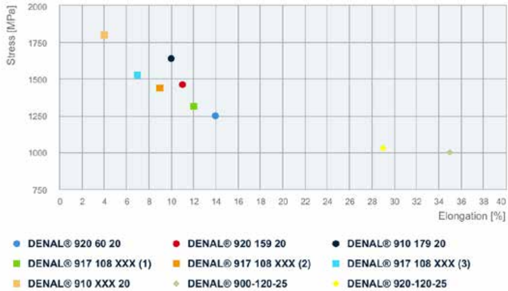
UTS Tensile strength of DENAL® (average values)
