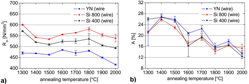
Figure 2: Results from tensile tests performed after heating up to a specific temperature followed by immediate cooling: a) Tensile strength; b) Fracture elongation
