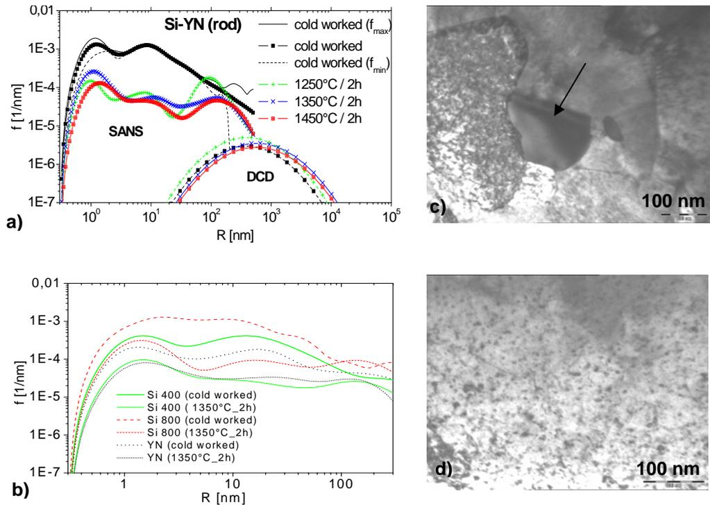
Figure 5: a) Particle size distributions of the Si-YN variant. (Samples prepared from  $6 \times 6$  mm<sup>2</sup> material.) b) Particle size distributions in samples Si 400, Si 800 and YN. c) TEM micrograph of a large Ta<sub>2</sub>Si precipitate (arrow) in the matrix (Si-YN sample, annealed for 30 minutes at  $830^\circ C$ ). d) TEM micrograph of fine particles in the matrix (Si 800 sample, annealed for 30 minutes at  $830^\circ C$ ).
