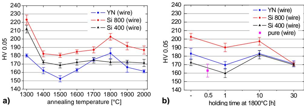
Figure 3: Microhardness (HV 0.05) of the tested wire samples. a) Samples heated up to the target temperature followed by immediate cooling. b) Samples annealed at 1800°C for different times.
