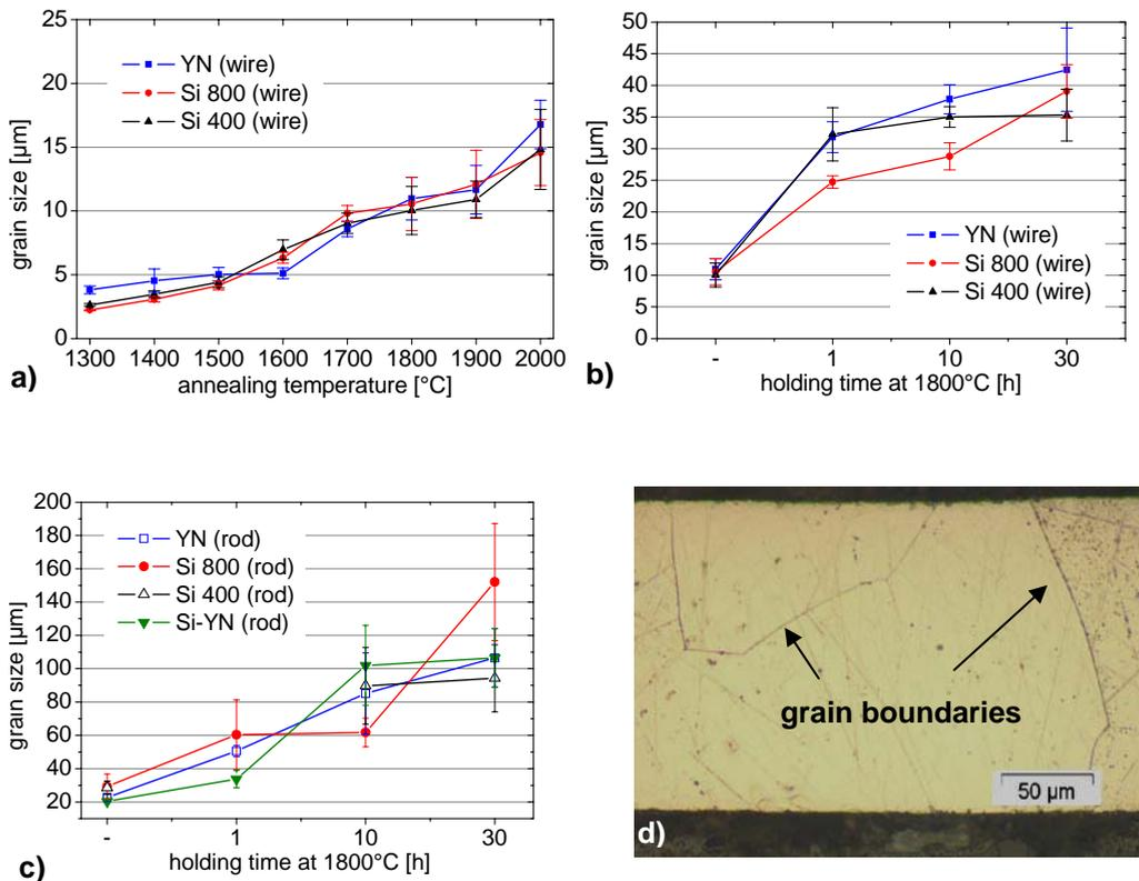
Figure 4: Average grain size of annealed samples. a) Wire samples heated up to target temperature indicated (no holding time). b) Wire samples annealed at 1800°C for different times. c) Samples prepared from 6x6 mm<sup>2</sup> rods and annealed at 1800°C for different times. The results derived from the Si-YN variant are included. d) Large grains in a wire made from pure Ta ingot and annealed at 1800°C for 30 minutes, LOM
