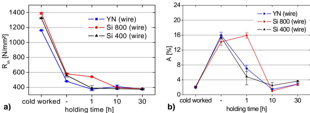
Figure 1: Results from tensile tests performed after cold working or annealing at 1800°C for different times: a) Tensile strength; b) Fracture elongation
