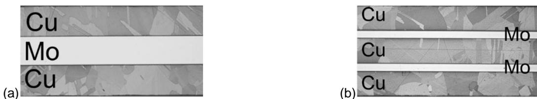
Figure 2: Polished cross sections of (a) a three and (b) five layered molybdenum-copper-composite.
