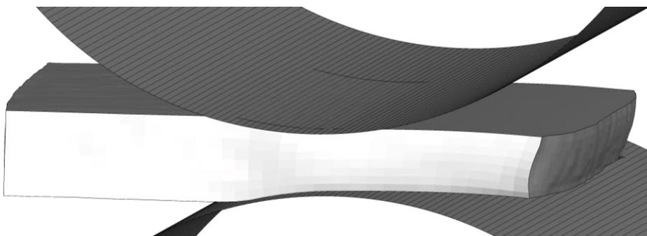
Figure 9: Simulation of hot rolling of a Mo plate.
