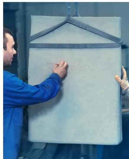
Figure 2: Mo green part after powder compaction.
