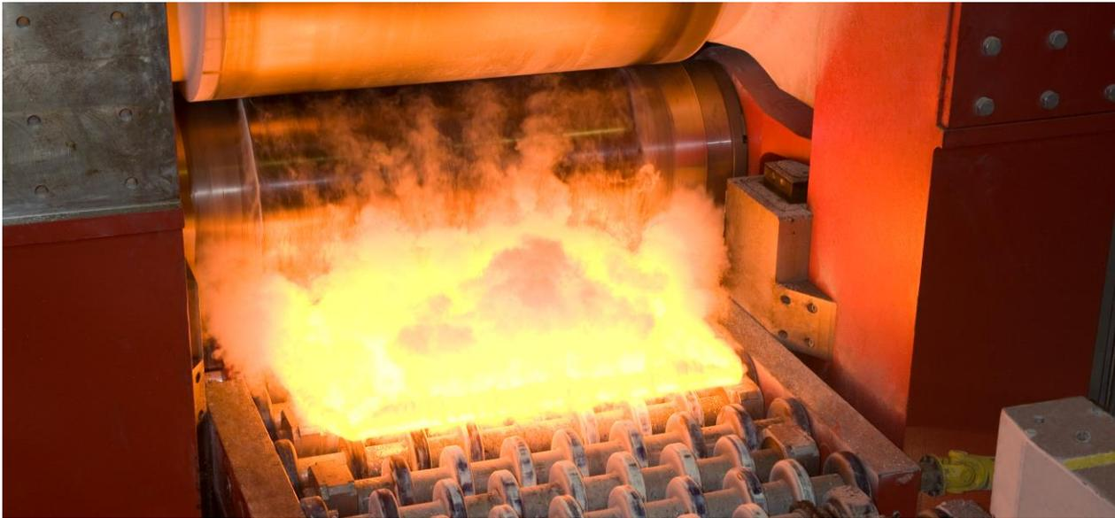
Figure 4: Hot rolling of a Mo plate.
